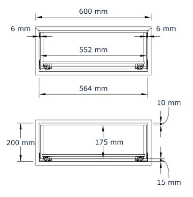
To calculate the width Internal aperture minus 12mm
