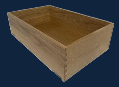
Our dovetail drawer boxes are made in our workshop in Yorkshire from the highest quality materials. 15mm stock, dovetailed joints with the 10mm base grooved all round, notched and drilled for undermount drawer runners. Available lacquered or raw finish.
